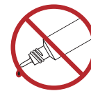
Angle incorrect de distribution
