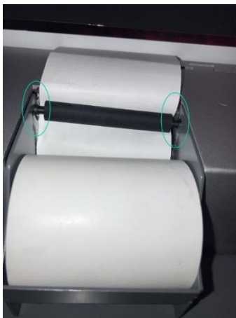
Figure 19 - printer paper replacement: pin off axis
