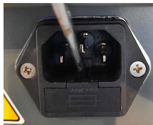
Figure 15 – Replacement of the fuses: extraction box
