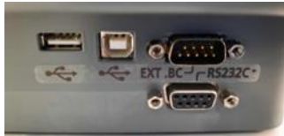
Figure 6 – Connectors for external supports
