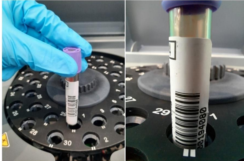
Figure 24 Correct insertion of the test tube
