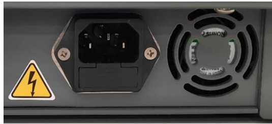
Figure 14 – Replacement of the fuses: fuses box
