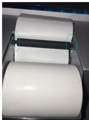
Figure 18 - Printer paper replacement: roll off axis
