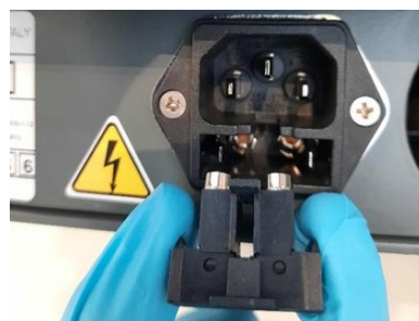
Figure 17 – Replacement of the fuses: repositioning box
