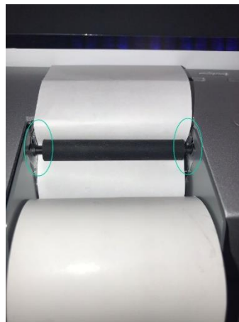
Figure 20 - Printer paper replacement: correct position
