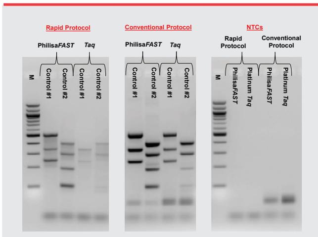
Agarose gel data, produced on the Philisa Thermal Cycler, following amplification of Philisa *ampC* ID kit controls using both rapid and conventional protocols with PhilisaFAST and wild-type *Taq* DNA polymerase, as per each enzyme's respective IFU guidelines. NTCs are indicated as a control for identification of contamination in PCR reaction mixes.
