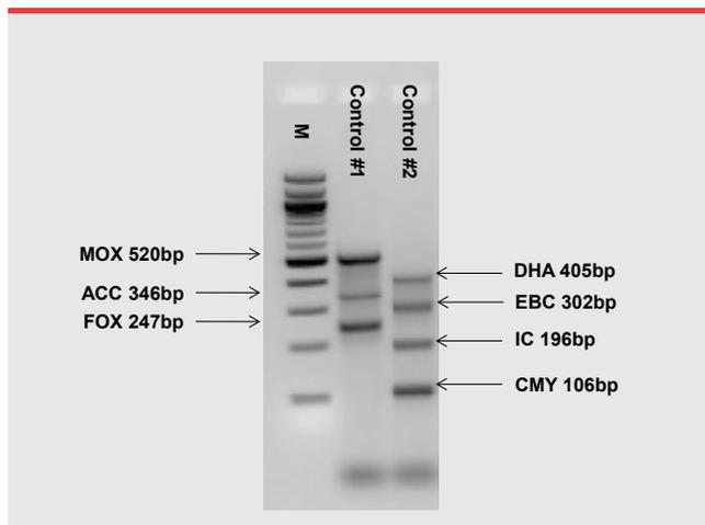
Agarose gel depicting Philisa *ampC* ID kit gel products following amplification of the kit DNA controls using the manufacturer's recommended protocol for rapid PCR with the Philisa Thermal Cycler and PhilisaFAST DNA polymerase to carry out the PCR. As indicated, control #1 gel products include MOX, ACC, and FOX *ampC* gene families. Control #2 gel products include DHA, EBC, internal control, and CIT gene families.
