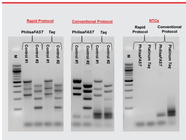
Comparison of PhilisaFAST and *Taq* DNA Polymerase amplification of the Philisa *ampC* ID kit controls using the Philisa *ampC* ID kit with both rapid and conventional PCR protocols. PhilisaFAST amplifications were according to the manufacturer's IFU. For amplifications with *Taq* polymerase, magnesium concentration was increased to 2 mM and DNA polymerase concentration was increased to 1.25 U per reaction. NTC samples are indicated as a control for contamination of reaction mixes.
