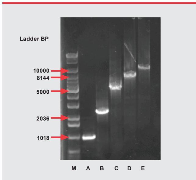
**IFU Based Protocol Gel** - the gel results of the initial IFU guided protocol for the Lambda Phage DNA long amplicon PCR. Well M is a molecular weight marker. Wells A, B, C, D, and E are 1, 2.5, 5, 7.5, and 10 kb amplicons, respectively. For gel analysis, 6  $\mu$ L of PCR product was loaded on a 0.7% gel and run at 70 V for 100 minutes. After electrophoresis, gel was stained with ethidium bromide and imaged on a molecular imager.
