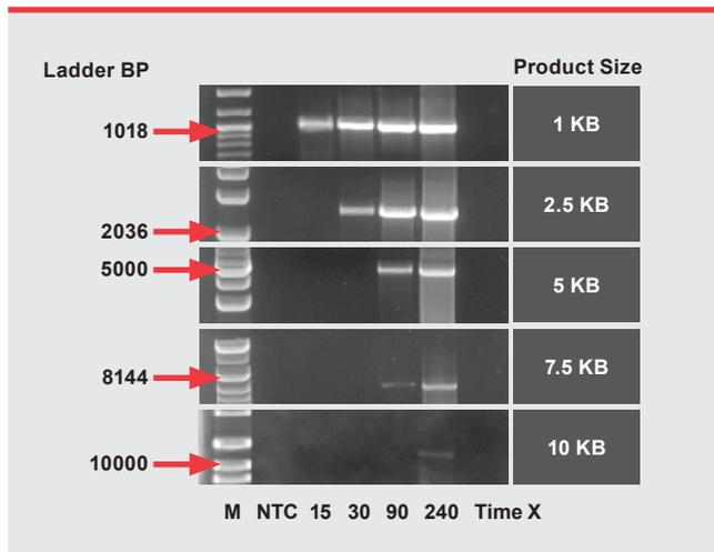
**Optimized Protocol Gel** – the gel results of the optimized protocol for the Lambda Phage DNA long amplicon PCR. The anneal/extension time is noted below the figure in seconds, with NTC (15-second protocol was used for NTCs). For gel analysis, 6  $\mu$ L of PCR product was loaded on a 0.7% gel and run at 70 V for 80-180 minutes depending on amplicon size. After electrophoresis, gels were stained with ethidium bromide and imaged on a digital imager.
